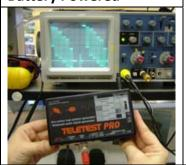
The TELETEST PRO is a high quality video test pattern and audio signal generator for use by engineers and AV technicians who deal with broadcast A/V products.
